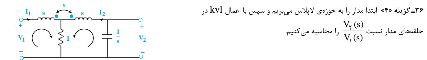
$$\text{KVL: } -V_1 + sI_1 + sI_\gamma + (I_1 + I_\gamma) = 0 \Rightarrow V_1 = (s+1)I_1 + (s+1)I_\gamma \quad (1)$$
