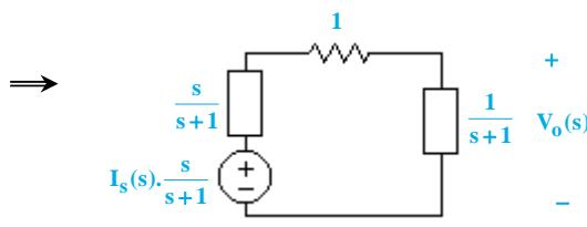
$$\Rightarrow V_o(s) = \frac{\frac{1}{s+1}}{\frac{1}{s+1} + 1 + \frac{s}{s+1}} \times \frac{s}{s+1} I_s(s) = \frac{1}{2} \times \frac{s}{s+1} I_s(s)$$
