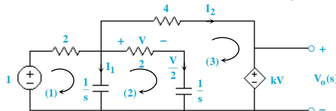
$$kvl(1): -1 + 2 \times (I_1 + I_2 + \frac{V}{2}) + \frac{I_1}{s} = 0 \Rightarrow (2s+1)I_1 + 2sI_2 + sV = s \quad (1)$$
