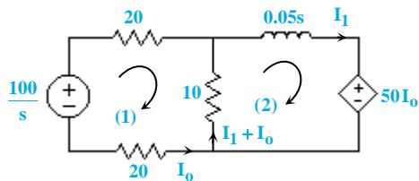
$$\left\{ \begin{array}{l} kvl(1): 50I_0 + 10I_1 = -\frac{100}{s} \\ kvl(2): (\frac{10}{20} \Delta s + 10)I_1 + 10I_0 = -50I_0 \Rightarrow I_1 = \frac{-60I_0}{10 + \frac{10}{20}\Delta s} \end{array} \right. \quad (1), (2)$$
