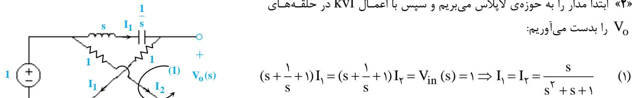
$$(s + \frac{1}{s} + 1)I_1 = (s + \frac{1}{s} + 1)I_2 = V_{in}(s) = 1 \Rightarrow I_1 = I_2 = \frac{s}{s^2 + s + 1} \quad (1)$$
