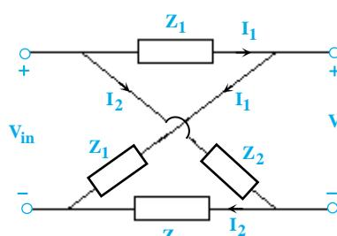
$$\underline{V_{in} = 2Z_1 I_1} = Z_2 I_2 + Z_4 I_4 \Rightarrow I_2 = \frac{2Z_1}{Z_2 + Z_4} I_1 \quad (۲)$$
