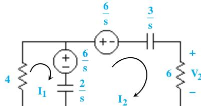
$$\text{KVL(۱)}: 6I_1 + \frac{6}{s} + \frac{2}{s}(I_1 - I_2) = 0 \Rightarrow (6s + 2)I_1 - 2I_2 = -6 \quad (۱)$$
