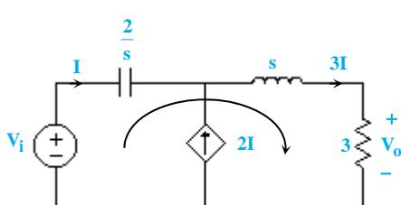
$$V_o = 3 \times 3I = 9I = \frac{9s}{3s^2 + 9s + 2} V_i \Rightarrow \frac{V_o}{V_i} = \frac{9s}{3s^2 + 9s + 2}$$
