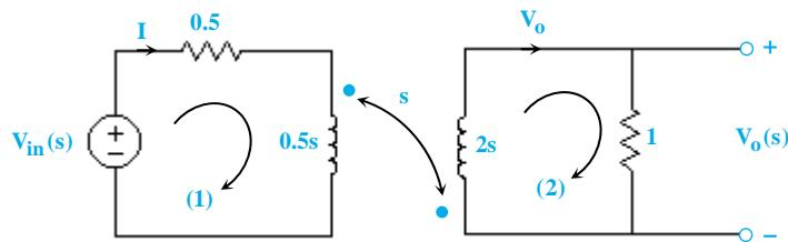
$$\text{kvl(1)}: -V_{in} + \circ / \Delta I + \circ / \Delta s I + s V_o = \circ \Rightarrow (s+1)I + 2sV_o = 2V_{in} \quad (1)$$
