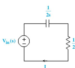
$$I(s) = \frac{V_{in}(s)}{\frac{1}{2s} + \frac{1}{2s}} = \frac{2s V_{in}(s)}{s+1}$$
