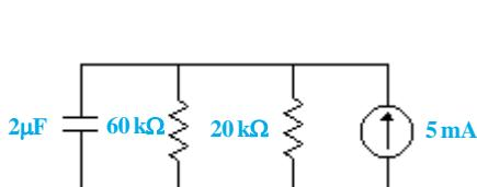
$$\begin{cases} v_C(\infty) = 5 \times 10^{-3} \times (20 \parallel 60) \times 10^3 = 75 \text{ V} \\ R_{eq} = 20 \parallel 60 = 15 \text{ k}\Omega \quad \Rightarrow \quad v_C(t) = 75 - 120 e^{-100t} \text{ V} \\ \tau = RC = 15 \times 10^3 \times \frac{2}{3} \times 10^{-6} = 10^{-2} \end{cases}$$
