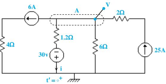
$$\begin{aligned} \text{KCLA: } & \frac{V + 3}{1/2} + \frac{V}{\delta} + \gamma - \Delta = 0 \Rightarrow V = -\gamma V \\ \Rightarrow i &= \frac{V + 3}{1/2} = 2 \text{ A} \\ \Rightarrow i(t' = 0^+) &= 2 \text{ A} \end{aligned}$$
