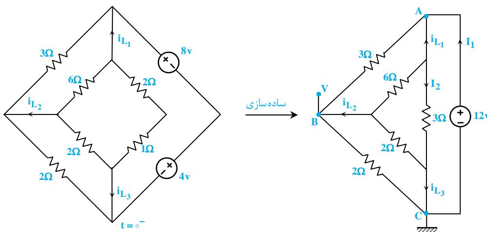
$$V = \frac{2 \parallel 2}{(2 \parallel 2) + (3 \parallel 6)} \times 12 = \frac{1}{3} \times 12 = 4V, \quad I_1 = \frac{12}{2 \parallel (2+1)} = \frac{12}{1/5} = 6A$$
