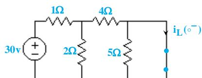
$$i_L(\circ^-) = \frac{2}{2+4} \times \frac{3^\circ}{1+(2||4)} = \frac{3^\circ}{4} A$$
