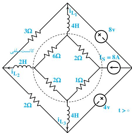
$$i_{L_1}(\circ^+) = \frac{L_{eq}}{L_1} \times [I_S - o] + i_{L_1}(\circ^-) = \frac{1}{\frac{1}{4} + \frac{1}{2} + \frac{1}{4}} \times 8 - \frac{1}{3} = \frac{1}{4} \times 8 - \frac{1}{3} = \frac{1}{3} A$$
