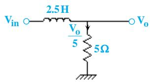
$$\begin{aligned} \text{KVL: } & -V_{in} + \frac{1}{5} \frac{dV_o}{dt} + V_o = 0 \\ & \Rightarrow \frac{dV_o}{dt} + 2V_o = 2V_{in} \end{aligned}$$
