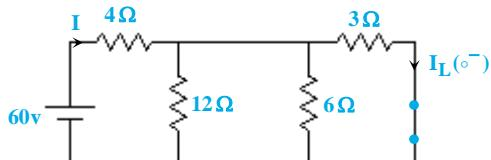
$$I = \frac{60}{4 + 12 \parallel 6 \parallel 3} = 10/5 \Rightarrow I_L(0^-) = \frac{12 \parallel 6}{12 \parallel 6 + 3} \times 10/5 = 6A$$
