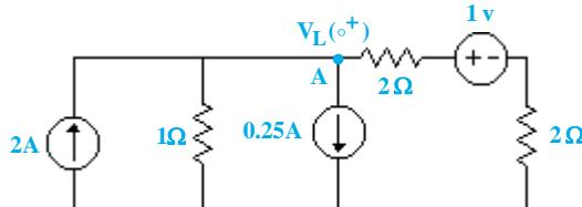
$$\text{KCL (A): } -2 + \frac{V_C(\circ^+)}{1} + 0.25 + \frac{V_C(\circ^+) - 1}{4} = 0$$
