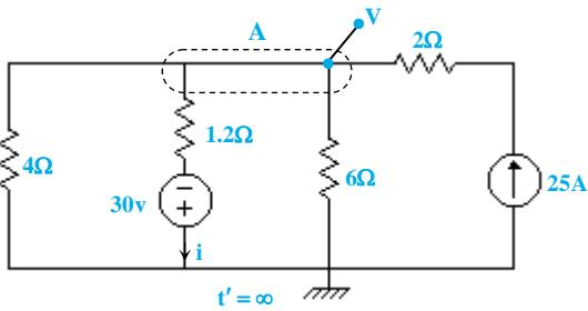
$$\begin{aligned} \text{KCLA: } & \frac{V}{\gamma} + \frac{V + 3}{1/2} + \frac{V}{\delta} - \Delta = 0 \Rightarrow V = 0 \\ \Rightarrow i &= \frac{V + 3}{1/2} = 2 \Delta \text{ A} \\ \Rightarrow i(t' = \infty) &= 2 \Delta \text{ A} \end{aligned}$$
