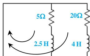
$$\begin{cases} I_r(t) = I_r(\infty) + (I_r(0) - I_r(\infty)) e^{-\frac{R_{eq_r} t}{L_r}} = 0/6 e^{-\Delta t} \text{ A} \\ I_l(t) = I_l(\infty) + (I_l(0) - I_l(\infty)) e^{-\frac{R_{eq_l} t}{L_l}} = 2/4 e^{-2t} \text{ A} \end{cases}$$
