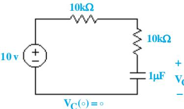
$$\begin{aligned} v_C(\infty) &= 10 \text{ V} \\ R_{eq} &= 10 + 10 = 20 \text{ k}\Omega \\ \tau &= RC = 20 \times 10^3 \times 10^{-6} = 0.2 \text{ sec} \\ \Rightarrow v_C(t) &= 10(1 - e^{-t/0.2}) \xrightarrow{t=13/8 \text{ ms}} v_C(13/8 \text{ ms}) = 10(1 - e^{-0/69}) = 5 \text{ V} \\ \Rightarrow v_C(13/8^+) &= v_C(13/8^-) = 5 \text{ V} \end{aligned}$$
