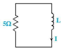
$$\begin{aligned} i_L(\infty) &= 0 \Rightarrow i_L(t) = i_L(\circ^+) e^{-\frac{R}{L}t} \\ \Rightarrow i_L(t) &= \frac{3^\circ}{4} e^{-\frac{\Delta}{L}t} \xrightarrow{i_L(\circ/1) = 1/14} 1/14 = 4/28 e^{-\frac{\circ/\Delta}{L}} \\ \Rightarrow \frac{\circ/\Delta}{L} &= \ln \frac{4/28}{1/14} \Rightarrow L = \frac{\circ/\Delta}{\ln 4/28} = \frac{-\circ/\Delta}{\ln 4/28} H \end{aligned}$$
