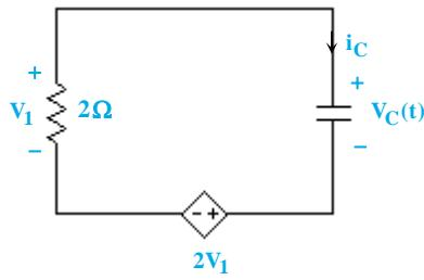
$$\begin{aligned} i_C(t) &= -\frac{v_1}{2} \Rightarrow \frac{dv_C(t)}{dt} = -\frac{v_1}{2} \\ &\Rightarrow \frac{dv_C(t)}{dt} = -\frac{1}{6} v_1 \quad (2) \\ \xrightarrow{(1),(2)} \frac{dv_C(t)}{dt} &= \frac{v_C(t)}{6} \Rightarrow \frac{dv_C(0^+)}{dt} = \frac{v_C(0^-)}{6} = \frac{-4}{6} = -\frac{2}{3} \end{aligned}$$
