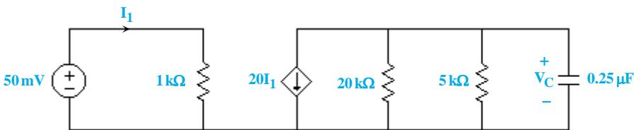
$$I_1 = \frac{50 \text{ mV}}{1 \text{ k}\Omega} = 50 \mu\text{A}$$
