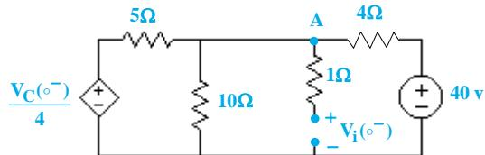
$$\text{KCL (A): } \frac{V_C(\circ^-) - 4}{4} + \frac{V_C(\circ^-)}{10} + \frac{V_C(\circ^-) - \frac{V_C(\circ^-)}{4}}{4} = 0$$
