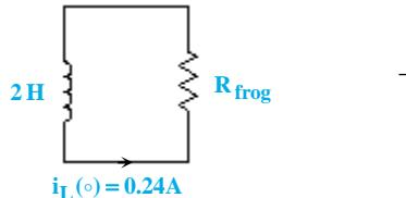
$$\xrightarrow{i_L(\infty) = 0} i_L(t) = i_L(\circ) e^{-\frac{R}{L}t} = 0.24 e^{-\frac{R}{2}t} \text{ A}$$
