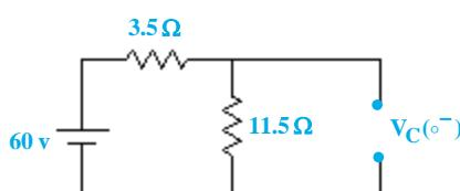
$V_C(\circ^-) = \frac{11/\Delta}{11/\Delta + 3/\Delta} \times 60 = 46 \text{ V}$
