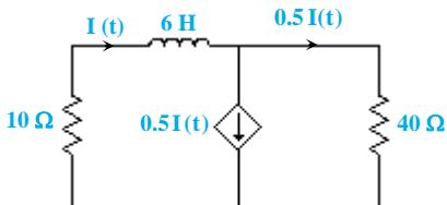
$$\begin{aligned} \tau^{-1} &= \frac{R_{eq}}{L} \\ R &= \frac{40 \times 0^+ / \Delta I(t)}{0^+ / \Delta I(t)} = 40 \Omega \Rightarrow R_{eq} = 40 \parallel 40 + 10 = 30 \Omega \\ \Rightarrow \tau^{-1} &= \frac{30}{6} = 5 \Rightarrow I(t) = 2e^{-5t} A \end{aligned}$$
