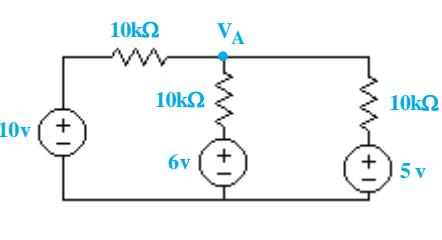
$$\begin{aligned} \frac{v_A - 10}{10} + \frac{v_A - 6}{10} + \frac{v_A - 5}{10} &= 0 \\ \Rightarrow 3v_A - 21 &\Rightarrow v_A = 7 \text{ V} \\ \Rightarrow I_C(13/8^+) &= \frac{7 - 5}{10 \times 10^3} = 0.2 \text{ mA} \end{aligned}$$
