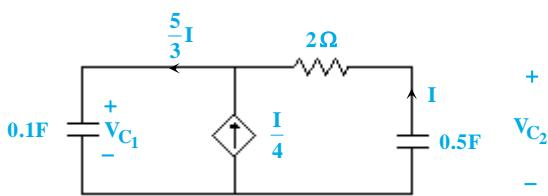
$$v_{C_1}(t) = v_{C_1}(0^+) + \frac{1}{0.1} \int_0^t \frac{5}{3} I dt$$
