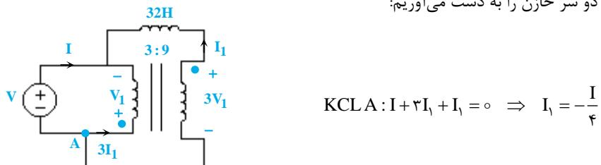
$$\text{KVL} : -V - 32 \frac{dI}{dt} + 3V_1 = 0 \xrightarrow{V_1 = -V} -4V - 32 \frac{d}{dt} \left( -\frac{I}{4} \right) = 0 \Rightarrow 4V = \frac{8dt}{dt} \Rightarrow V = \frac{2dt}{dt} \Rightarrow L_{eq} = 2H$$
