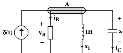
$$KCLA: -\delta(t) + i_R + x_1 + i_C = 0 \xrightarrow{(2),(3)} -\delta(t) + \frac{1}{x_2} + x_1 + \omega x_2 = 0 \Rightarrow \dot{x}_2 = -\frac{1}{\omega x_2} - \frac{x_1}{\omega x_2} + \delta(t) \quad (4)$$
