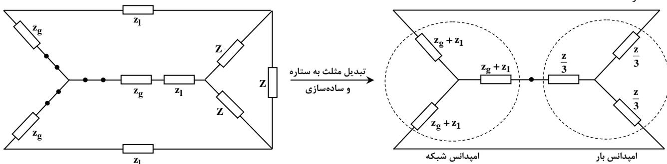
$$\frac{Z}{3} = (Z_g + Z_1)^* \Rightarrow Z = 3 \times (\omega / \omega + j\omega / \omega + \omega / \omega + j\omega / \omega)^* = 3 \times (1 + j\omega / \omega)^* = (3 - j1 / \omega) \Omega$$
