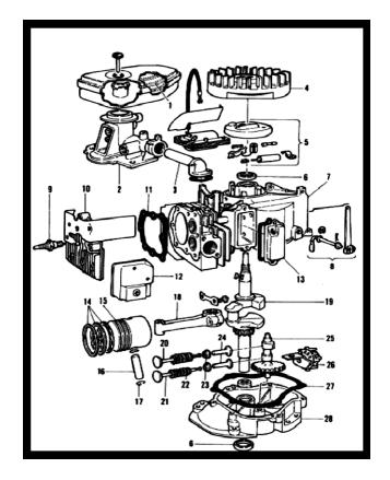
1. Air filter-prevents the entrance of dirt and other debris that will damage the engine if unfiltered.
