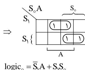
$$\text{logic}_0 = \bar{S}_1 A + S_1 S_0$$
